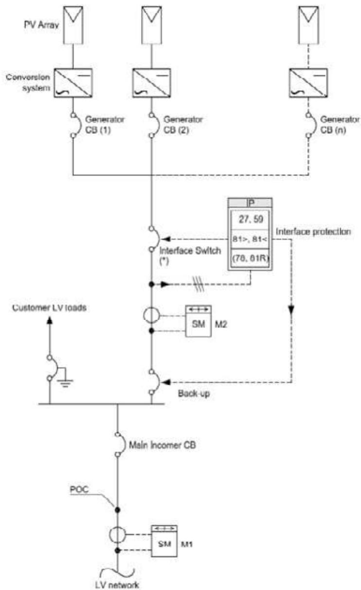
(\*) Motorized CR operated by undervoltage release or Contactor
