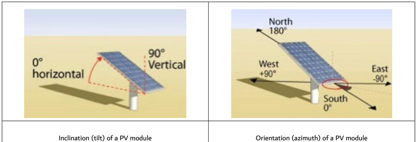
Figure 1 – Orientation and inclination of the PV panels
